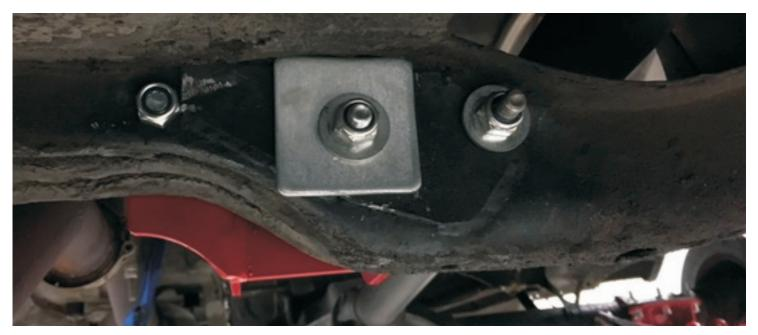
Reinforce the back of the beam as much as you think it is needed. Use supplied reinforceplate on the inside of the car
