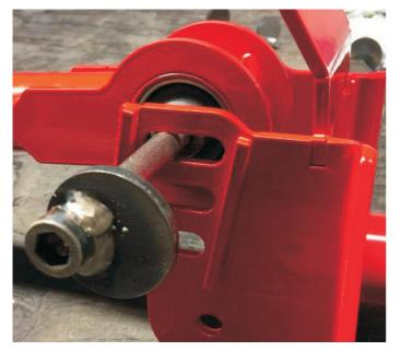
Install the upper strut in the top slot with the specialbolt
