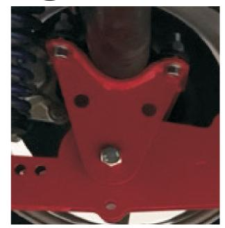
Weld the plate on the rear axel with 4 x 1cm long weld
